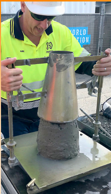
Concrete slump test demonstration by Hanson Concrete's Alex Kovac for apprentices.
